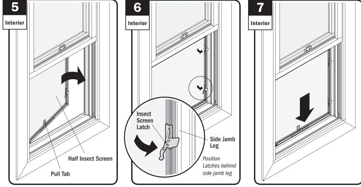
Rotate insect screen in using pull tab and latches.
