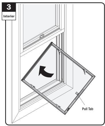
Hold sides near bottom of insect screen and pass through window opening.
