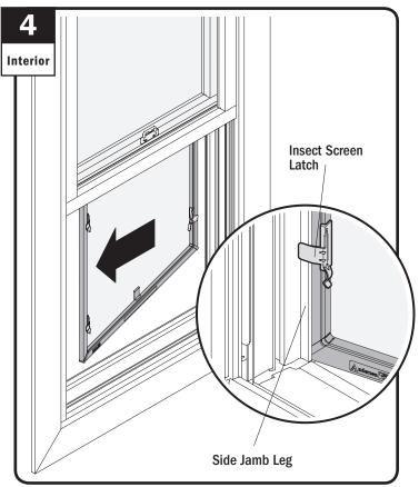
Push side with closed latches into side jamb. Position latches behind leg, as shown, creating a hinge point.
