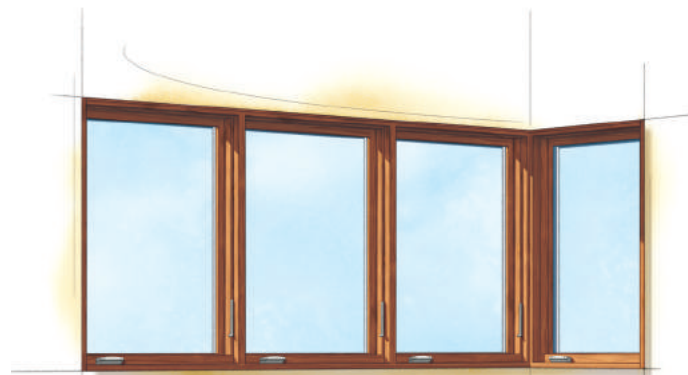
Casement and auxiliary window combination (interior)
