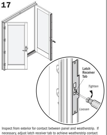
and compression using a flat blade screwdriver.
