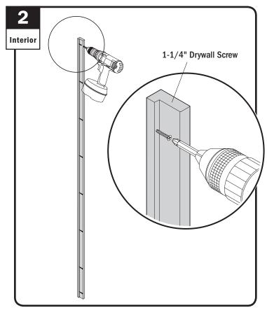
Start screws in all drilled holes.
