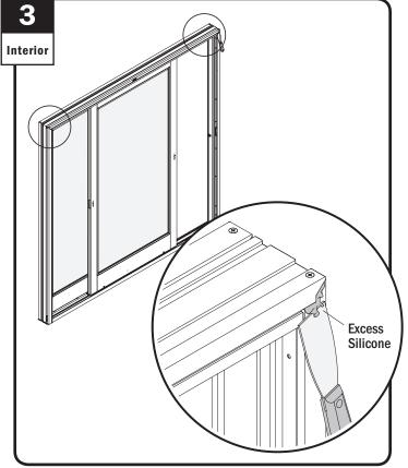
Open panel. Remove excess silicone from interior frame corners.
