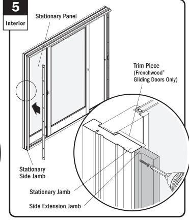
Position side extension jamb on stationary side jamb, flush with inside surface, and fasten using 1-1/4" screws. For Frenchwood Gliding Doors, **do not** flush with surface of trim piece.
