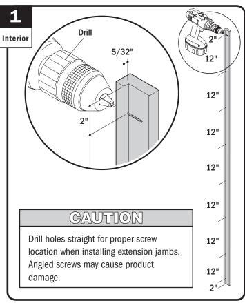
Drill 1/8" holes 2" from each end and every 12" in between on head and side extension jambs as shown.
