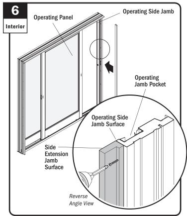
Position side extension jamb on operating side jamb, flush with inside surfaces, and fasten using 1-1/4" fasteners. Keep fasteners straight to avoid operating jamb pocket.
