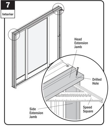
Square extension jamb ends at corners. Drill 1/8" hole and fasten using 1-1/4" screws as shown. **Installation is finished.**
