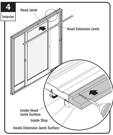
Center head extension jamb on head jamb. Keep inside jamb surfaces flush. **Do Not** overlap inside stop. Fasten extension jamb using 1-1/4" screws.
