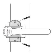
4. Pilot drill 1/8" x 1" deep holes and secure base plate to sash using No. 8x1" wood screws provided. Reset excutcheon plate to upright position. Assembly is complete.
