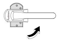
2. Align handle assembly over locking hardware shaft.
